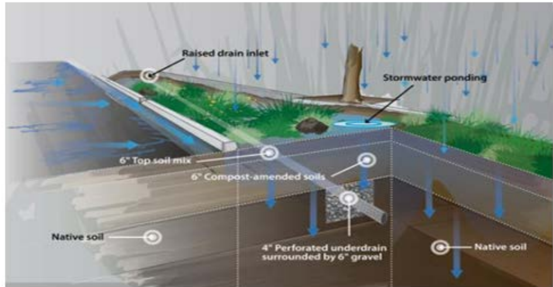
Figure B: Generic Urban Infiltration Trench Detail
