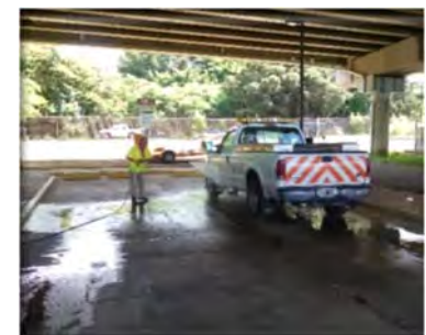
Wash vehicles within containment.
