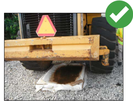
If a leak is observed, immediately place a drip pan or drip pad under the vehicle until repairs can be made.
